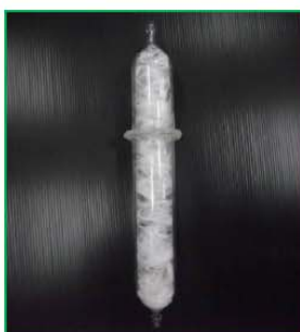
Figure 2. Experimental glass column containing fiberglass coated with catalyst.
