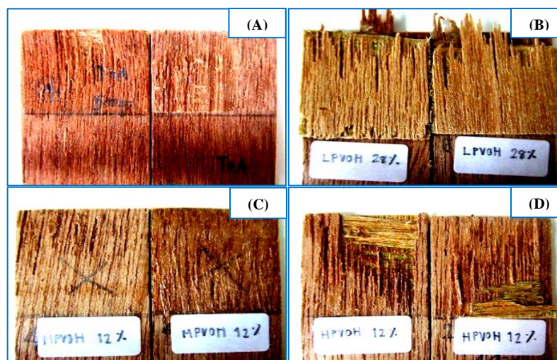
Figure 24. Photographs of the failure of commercial and PVOH adhesives joints at various types and concentrations. Commercial adhesive (A), L PVOH 28 wt% (B), M PVOH 12 wt% (C) and H PVOH 12 wt% (D), respectively.
