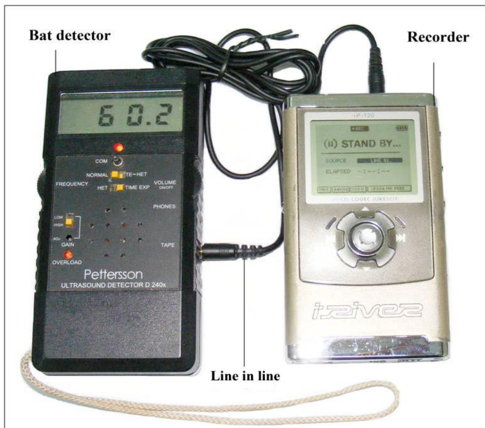
Figure 10. Bat detector connected with recorder.
