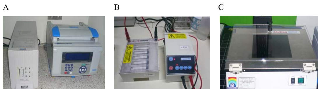
Figure 11 Takara PCR thermal cycler dice TP600 (Takara, Japan) (A), running gel electrophoresis (B) and UV light box (Gel Doc model 1000, Bio-Rad, USA) (C).
