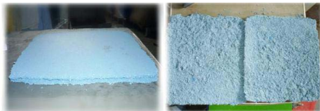
Figure 85. Composite panel from pilot scale prepared by 3% pMDI.
