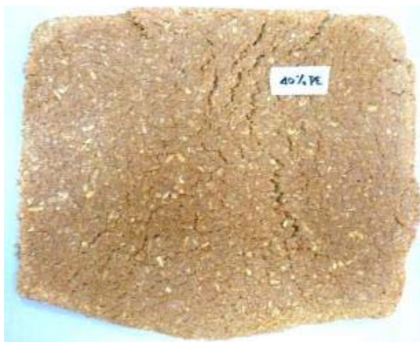
Figure 68. The appearance of composite panel prepared by using 40% Polyethylene as an additive.
