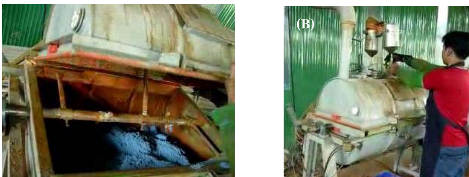
Figure 49. Mixing process of composite materials in pilot scale: (A) Inside mixing tank and (B) Outside mixing tank.
