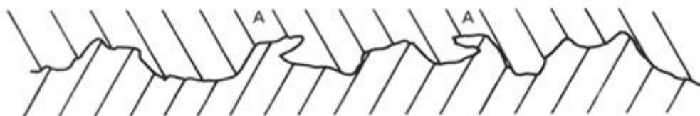
Figure 20. Reinforcement-Matrix Interface: Mechanical bonding.
