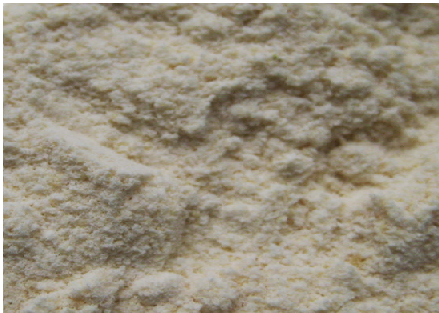
Appendix figure 3. soymilk residue with a sizes ranged from 20 mesh to 40 mesh
