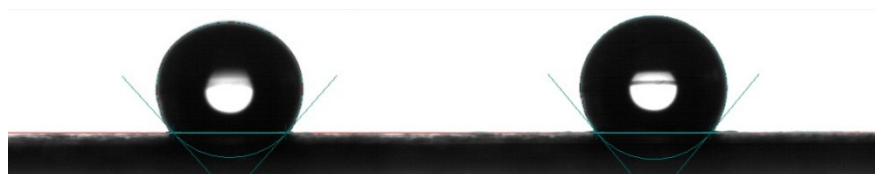
Figure 58. Contact angle of papersheets adding 7.5% caionic starch and 2.5% ASA of 0 and 1 minutes.
