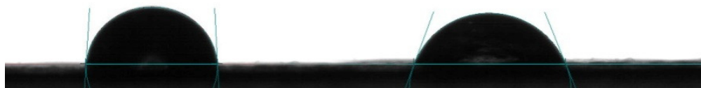
Figure 50. Contact angle of mixed pulpsheets made from Peach cedar and Cattail pulps in the ratio of 50:50 for 0 and 1 minutes.
