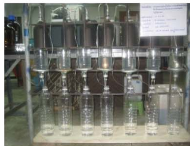
Fig. 1. Experimental set-up of batch reactors
