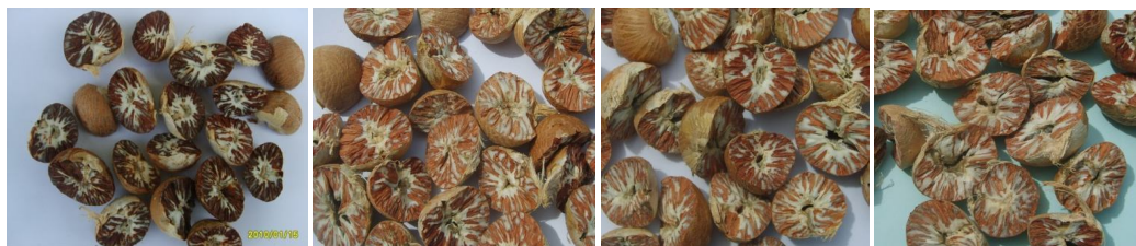
(ก) Sun dried (ข) Solar drying (ค) Biomass drying (ง) Solar and Biomass drying
