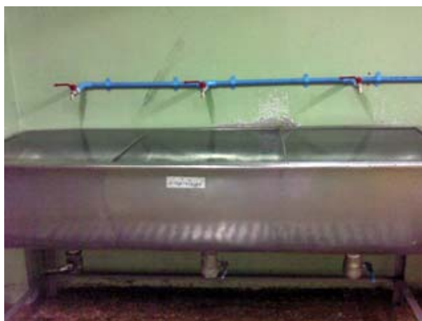
Figure 12. Sink for cleaning ice-cream bar molds after improvement
