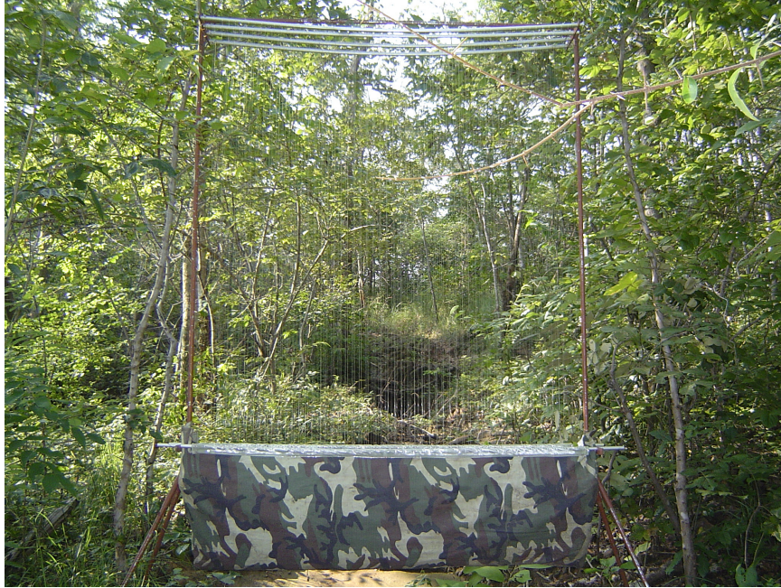
Figure 8. The harp trap was set across the nature trail in Phu Pha San, Phu Si Than Wildlife Sanctuary which surrounded by mixed deciduous forest.
