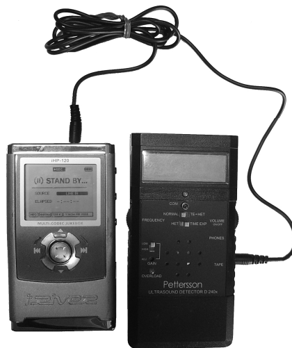
Figure 14. Pettersson ultrasound detector D 240x in time-expansion (10x) mode, connected to sound recorder i-RIVER model: iHP-120 Multi-codec jukebox
