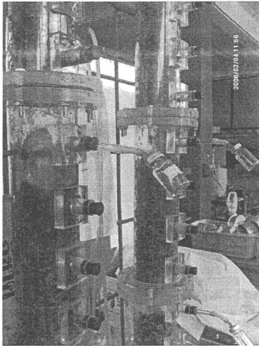
Figure 2-10 Collecting the gas sample.
