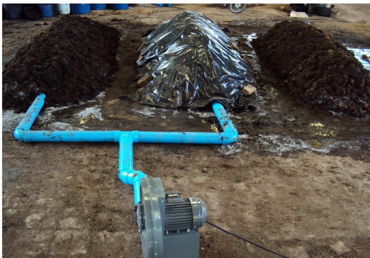
Figure 11. Characteristics of three aeration systems of compost from the palm oil mill wastes
