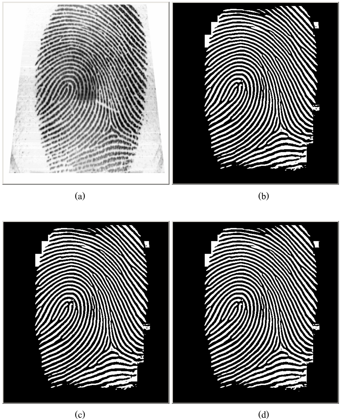
Figure 3.9. Result of the fingerprint image manipulated by a Gabor filter with different \delta_x and \delta_y values: (a) original gray scale fingerprint of good quality; (b) after filtered with of \delta_x and \delta_y of 12; (c) after filtered with of \delta_x and \delta_y of 20; (d) after filtered with of \delta_x and \delta_y of 30.
