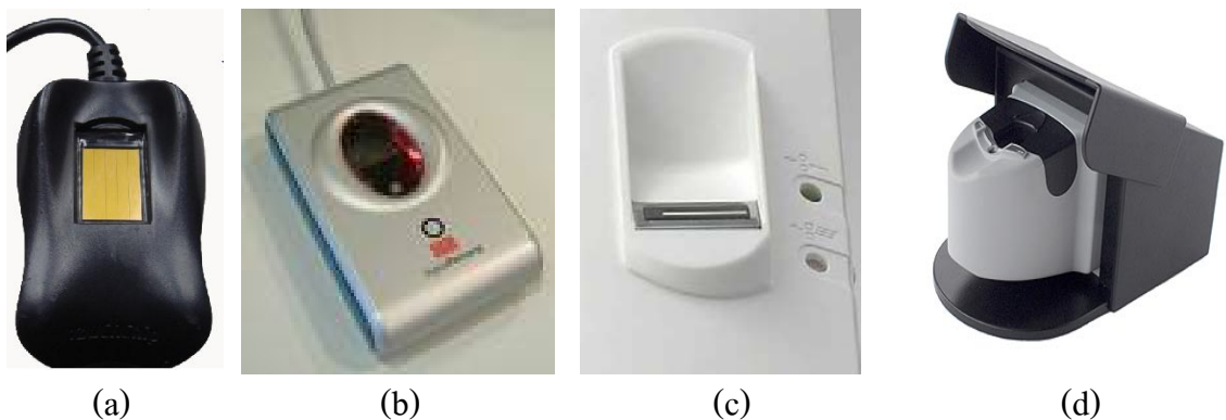
Figure 2.7. Four different types of fingerprint sensor;
