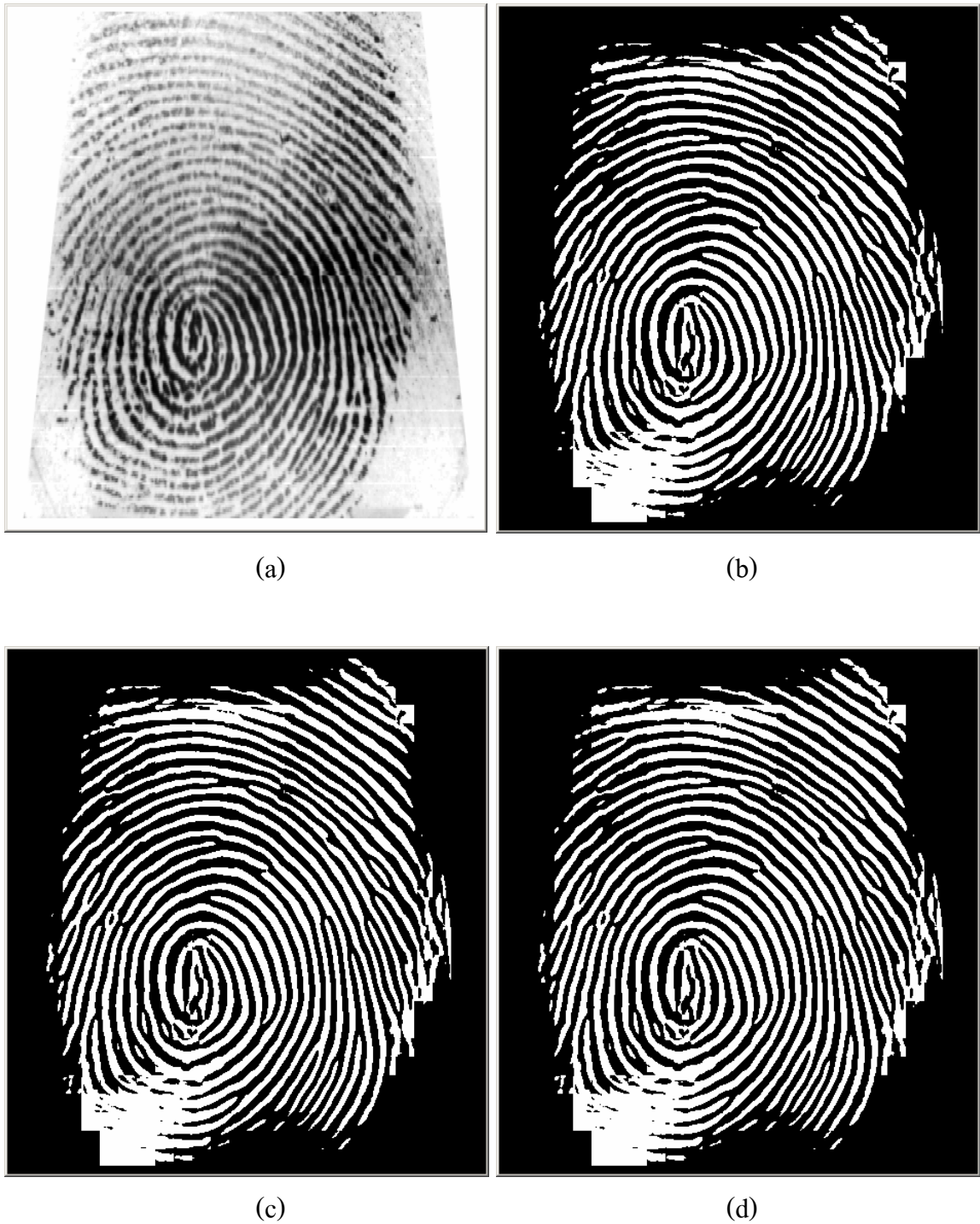
Figure 3.11. Result of the fingerprint image manipulated by a Gabor filter with different \delta_x and \delta_y values: (a) gray scale fingerprint of non-uniform pressure of the finger; (b) after filtered with of \delta_x and \delta_y of 12; (c) after filtered with of \delta_x and \delta_y of 20; ; (d) after filtered with of \delta_x and \delta_y of 30.
