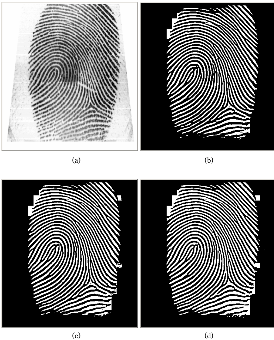
Figure 3.12. Result of the binarized fingerprint image due to different threshold values: (a) original gray scale fingerprint of good quality; (b) after binarized using threshold value of -800; (c) after binarized using threshold value of -400; (d) after binarized using threshold value of 0.
