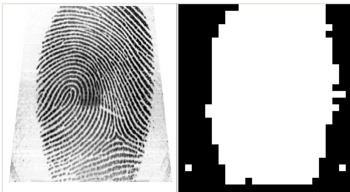
Figure 3.8. The fingerprint image (left) and the obtained minutiae mask image (right).
