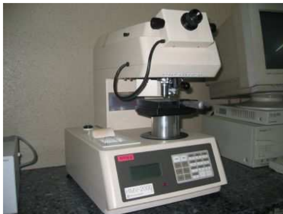
Figure 17. Vicker's surface hardness testing machine (Micromet II ,Buehler Ltd., Illinois, USA.)
