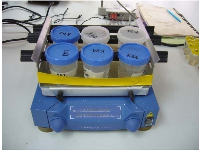
Figure 48. The each calvarial specimen was decalcified in 10% formic acid and agitated at 160 rpm on an orbital shaker (KS 130 Basic Orbital Shaker).
