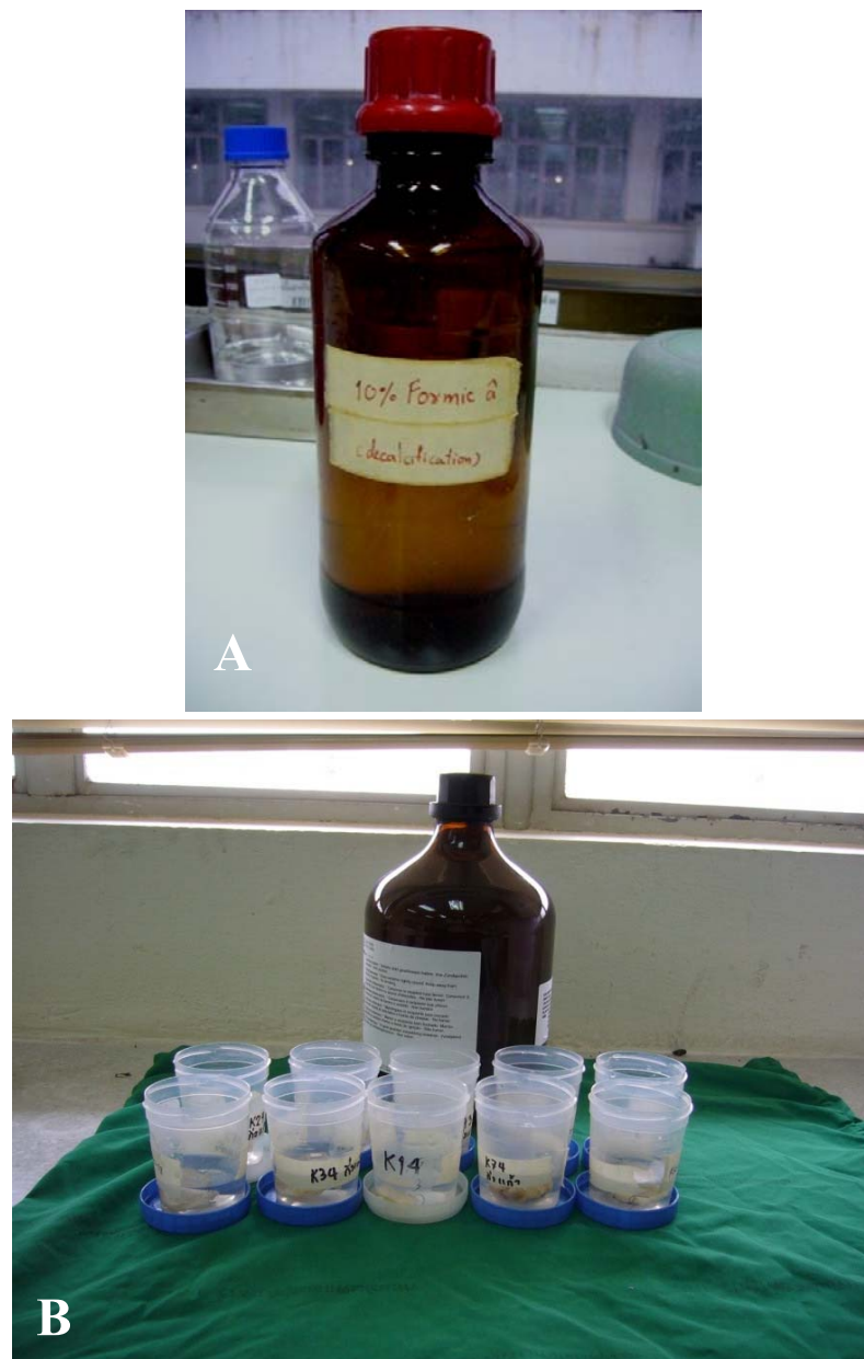
Figure 47. Decalcification was performed by using acid decalcifying agent, 10% formic acid (A). 10% formic acid was changed daily day for 3 weeks (B).
