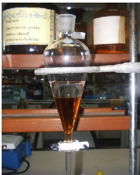
Figure 3-2 Two phases (organic and aqueous phase) separation after extraction using organic solvents
