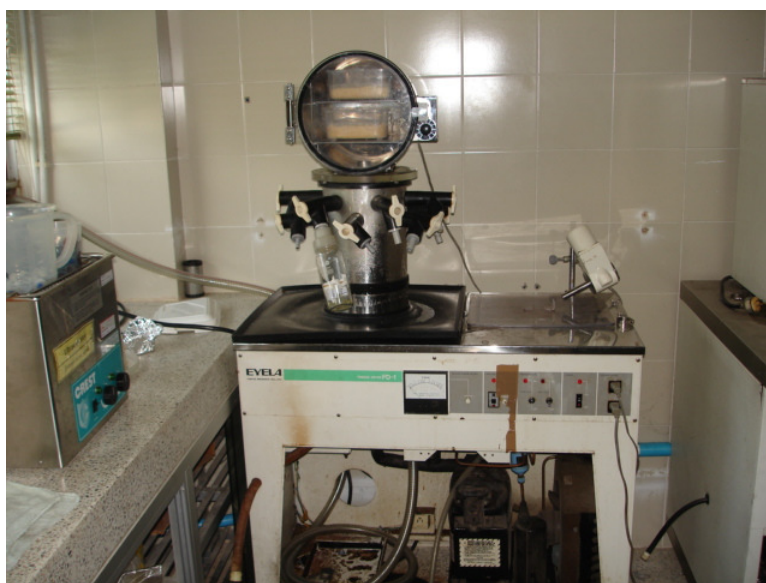
Figure 3-1 Freeze-dryer Eyela FD-1 (Rikakikai, Tokyo)
