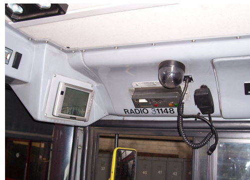
Radio and CCTV camera and monitor
