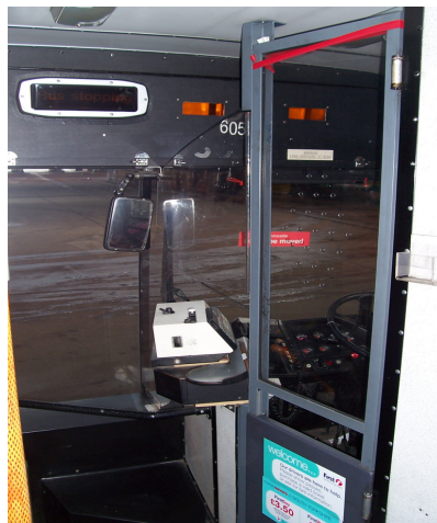
Cab door screen with retrofit extension
