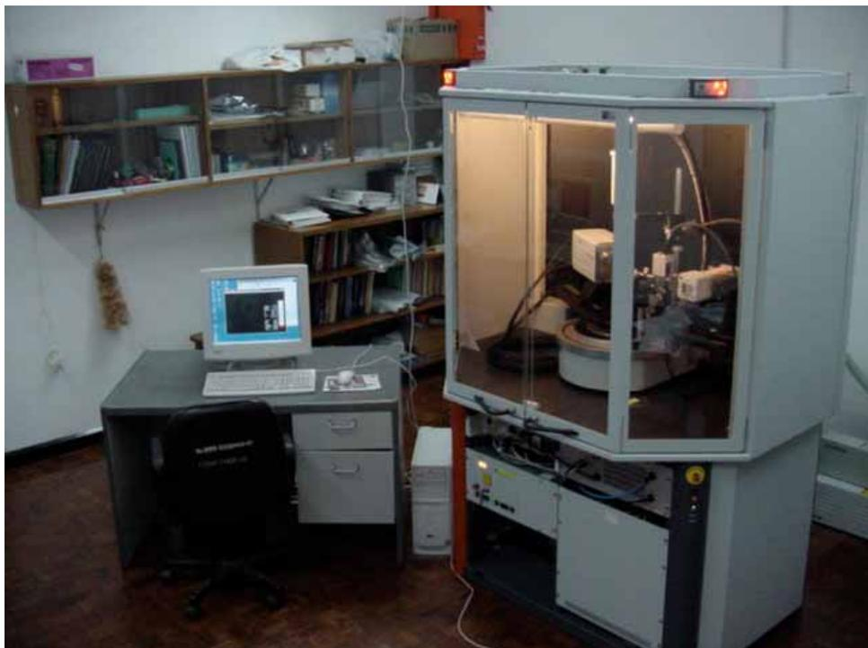
Figure 11 The SMART APEX CCD X-ray diffractometer.
