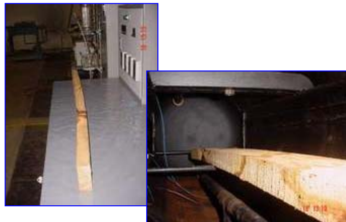
Figure B-2 After drying with superheated steam at 110°C for 36 hours, showing wood warp that develops during drying.
