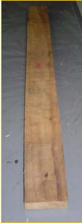
Figure B-16 Showing the straight wood after drying because wood was placed on the clamped rack support inside the chamber.
