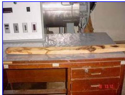
Figure B-4 The coffee-brown stains that develop during the superheated steam drying.
