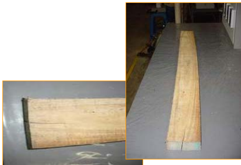
Figure B-13 The end check after drying.
