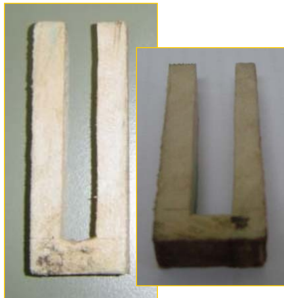
Figure B-17 Prong test showing acceptable piece of wood.
