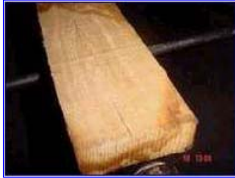
Figure B-3 Showing the end check after drying, end checks occurred in the wood rays, but on end-grain surfaces. End checks occur because moisture moves much faster in the longitudinal direction than in either transverse direction. There, the ends of boards dry faster than the middle and stresses develop at the ends (Simpson et al., 1991).
