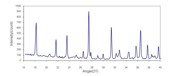
Sample identification: NaY(std) Start angle [ $^{\circ}2q$ ]: 16.280 End angle [ $^{\circ}2q$ ]: 40.880 Start d-value[Å]: 6.31731 End d-value[Å]: 2.56133 Maximum number of counts : 841 Anode material : Co A1 Wavelength [Å] : 1.78897 A2 Wavelength [Å] : 1.79285 Intensities for FIXED slit Peak positions defined by : Minimum of 2 nd derivative of peak Minimum peak tip width : 0.00 Maximum peak tip width : 1.00 Maximum peak base width : 2.00 Minimum significance : 0.75 Number of peak: 15
