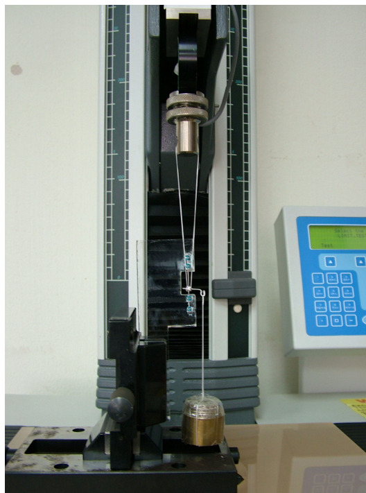
Fig. 1 An Instron testing machine, which measured the friction between bracket and archwire.
