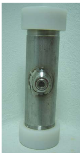
Figure 7. Diffusion cell for migration test of antimicrobial agents from coated paper
