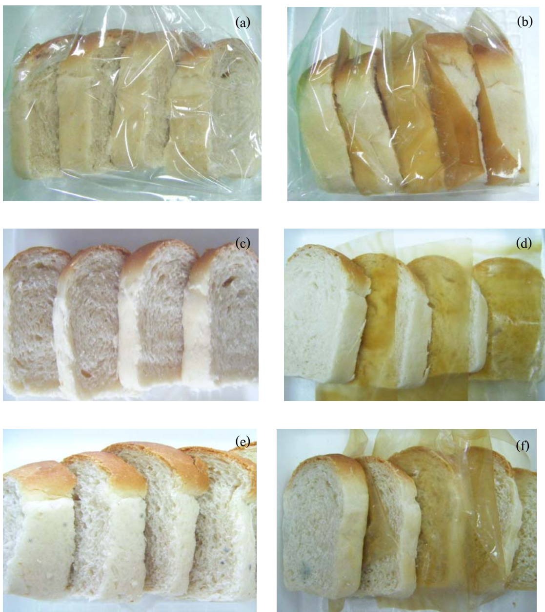
Figure 31. Illustrative pictures of sliced bread with no film (a), sliced bread applied with HPMC film incorporated with encapsulated clove extracts (b) at 0 day of storage and sliced bread applied with not film (c) and sliced bread applied with HPMC film incorporated with encapsulated clove extracts (d) at 2 days of storage and sliced bread applied with not film (e) at 4 days of storage and sliced bread applied with HPMC film incorporated with encapsulated clove extracts (f) at 6 days of storage, respectively.
