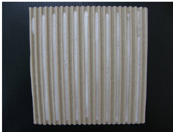
Figure 27. Coated paper with encapsulated orange aroma oil (80MD).
