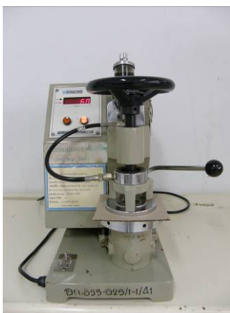
Figure 36. Test apparatus of bursting strength.
