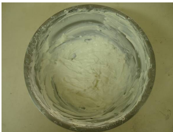
Figure 14. Appearance of encapsulation by paste method for 1:1 of wall material to orange aroma Ratio.
