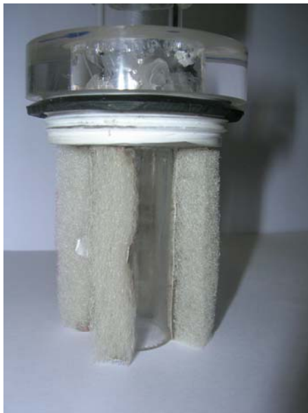
Figure 3.3 Photograph of cyclone combined with fibrous filter.
