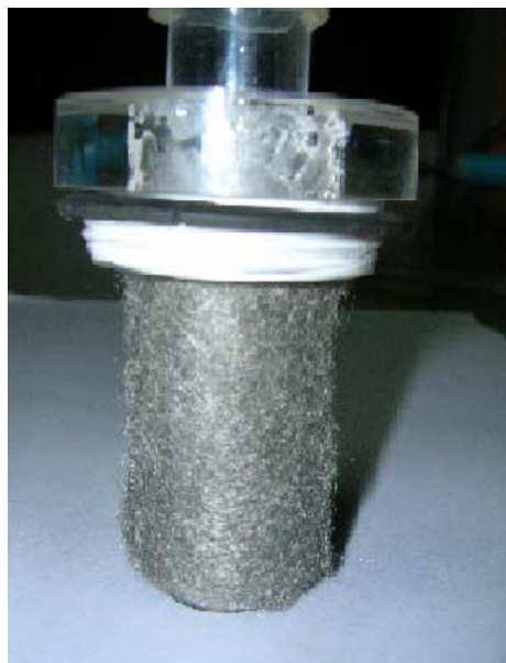
Figure 3.5 Photograph of cyclone combined with stainless steel filter.
