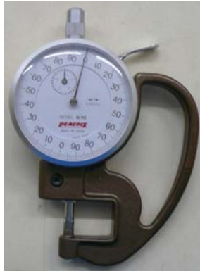
Figure 3.8 Thickness gauge handing.
