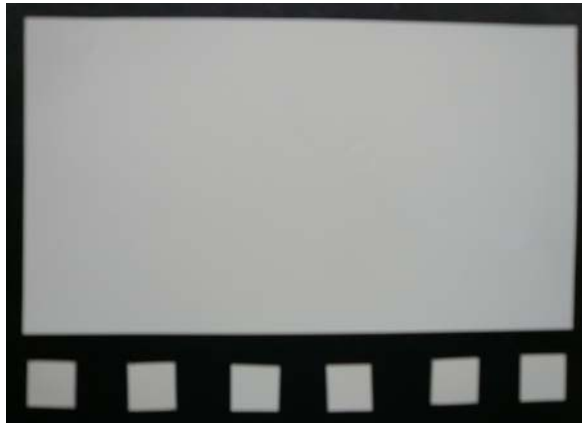
Figure 4.1 Pictorial view of a composite tape (upper) which was cut into pieces with dimensions of about 10 \times 10 \text{ mm}^2 (lower).
