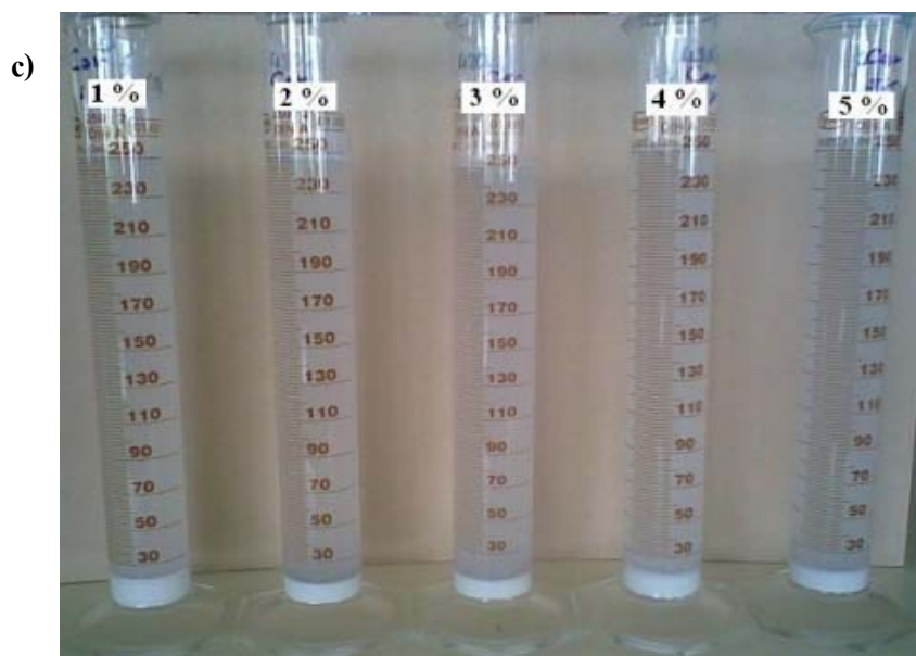
Figure 20. Effect of a) Locust bean gum, b) Xanthan gum and c) Carrageenan at various concentrations on the stability of alkyd resin coating (Cont.).
