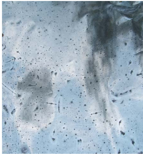
Figure 3.18 Erosion of OPP/MPET/LLDPE packaging of garcinia Tom-Yum paste after storage for 30 day
