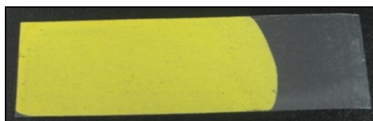
Figure 3.1 Uranium screen composed of Ammonium diurate [(\text{NH}_4)_2\text{U}_2\text{O}_7] .
