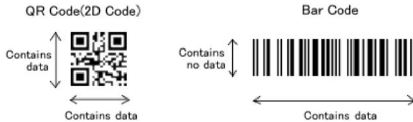
Figure 2.2 Comparison of QR code with traditional bar code
