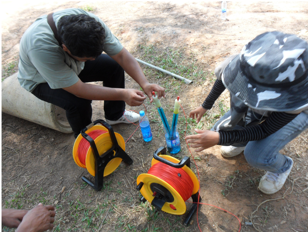
Figure 3.3 Preparing Cu-CuSO 4 electrodes for IP& resistivity and SP surveys
