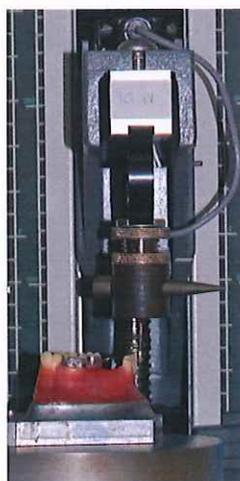
**Fig. 2:** Universal testing machine and testing method of asymmetrical V-bend
