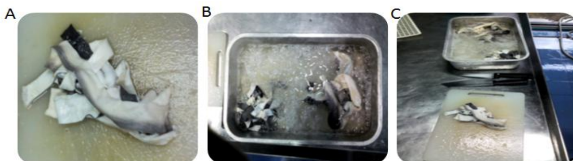
Figure 3.3 A. The frozen skin (-20 °C) was washed with cool water. B. Removed remaining meat on shark skin. C. Cut into small pieces (1.0*1.0 cm 2 ).
