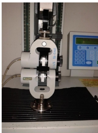
Figure 3.16 Universal testing machine (Lloyd instruments, LRX-plus, AMETEK Lloyd, instrument Ltd, Hampshire, UK) from Faculty of Dentistry, Prince of Songkla University.
