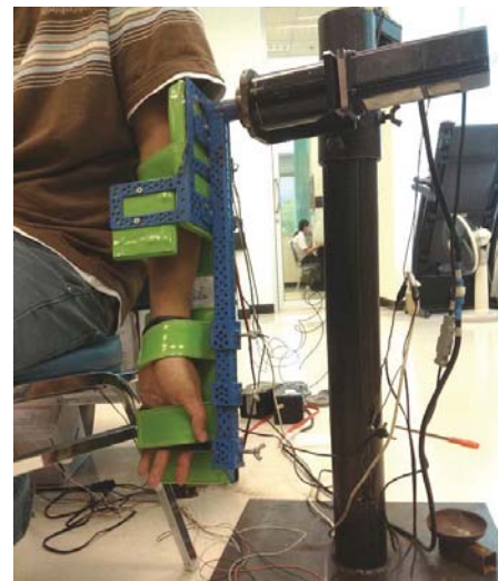
Fig. 5. Rehabilitation system for triceps muscle with hand and arm tourniquet device (for patient who cannot grip the hand).
