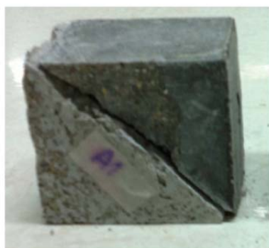
FIGURE 3: Slant shear sample after failure in compression test.
