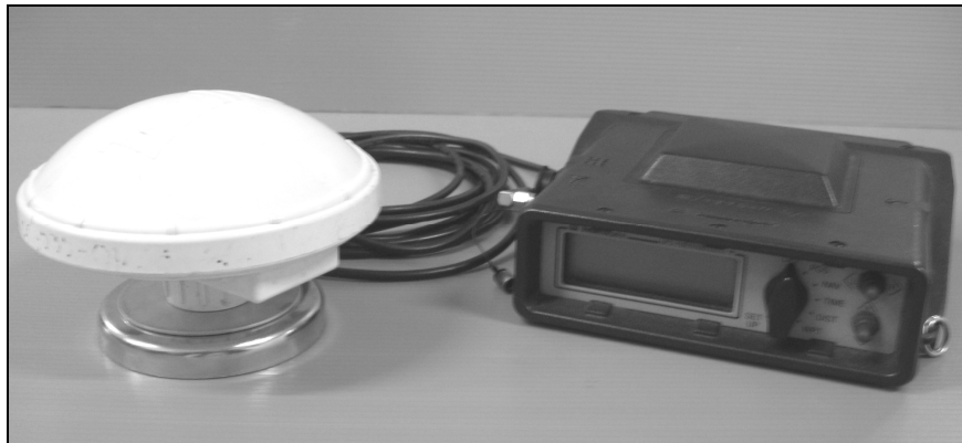
Figure 2.2 Trimble Basic Pathfinder GPS
