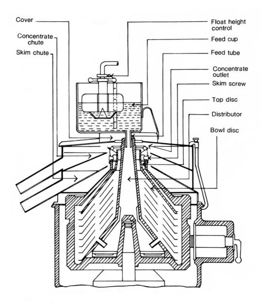
Fig. 7 A typical Alfa-Laval centrifuge bowl assembly.
