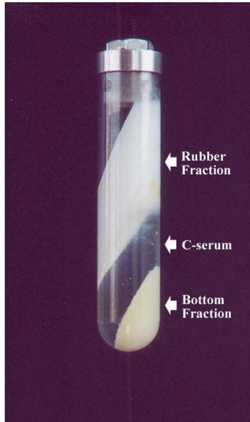
**Fig. 10** Ultracentrifugation of fresh latex.
