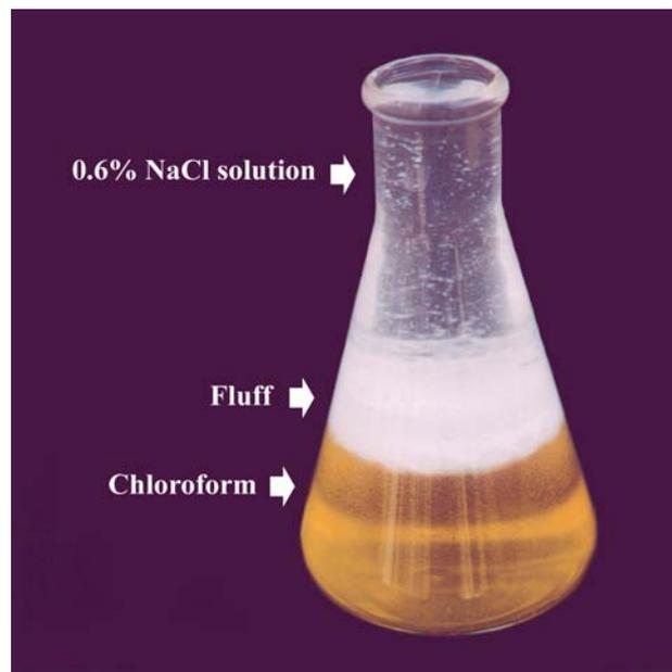
**Fig. 12** BFM fluff after washing with distilled water containing 0.6% NaCl for 48 h.
