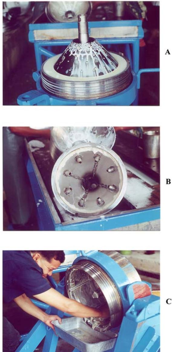
**Fig. 14** Remaining latex serum (A) and sludge (Band C) within the bowl casing of centrifuge.
