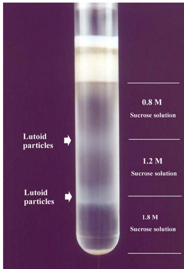
**Fig. 11** Separation of purified lutoid particles from fresh latex by centrifugation on discontinuous sucrose density gradients.
