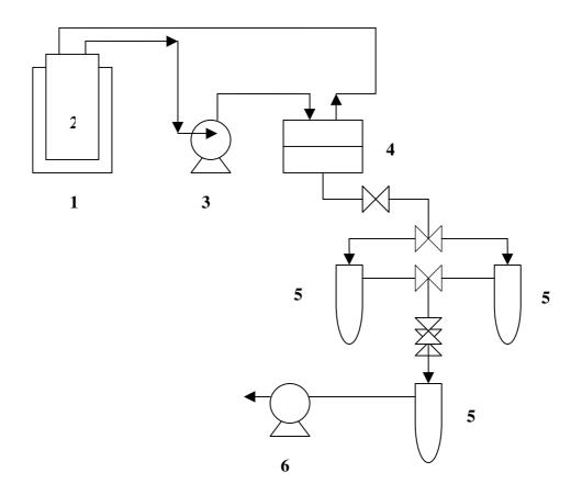
Figure 3.3 Schematic diagram of pervaporation setup, 1: heating mental, 2: feed tank, 3: feed circulation pump, 4: permeation cell, 5: cold trap and 6: vacuum pump.
