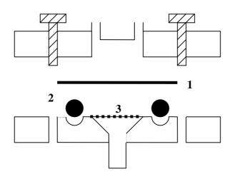
Figure 3.2 Schematic diagram of cross-section of permeation cell, 1: membrane,2: o-ring and 3: porous steel plate.
