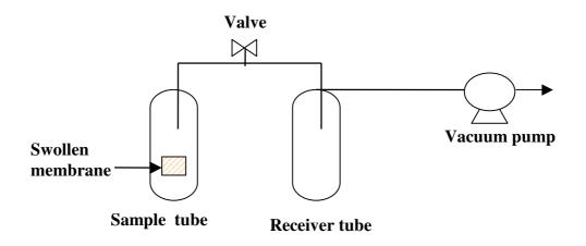
Figure 3.1 Schematic diagram of sorption apparatus.
