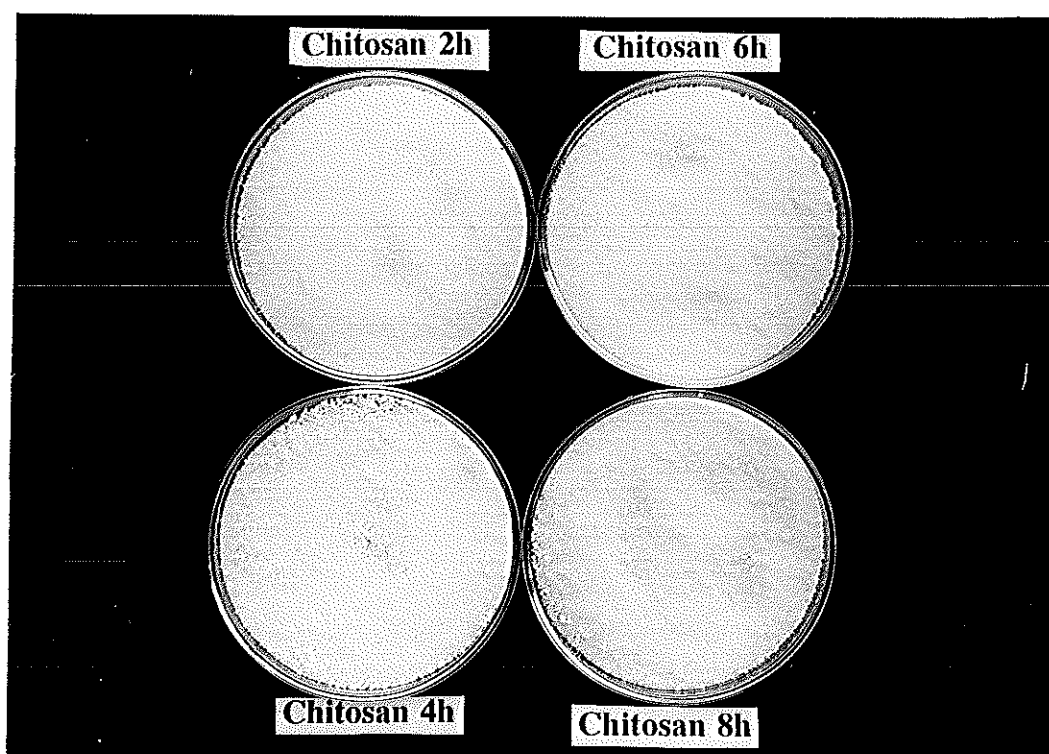
Figure 3.3 Appearance of chitosan prepared from a powder (0.75 mm) of squid pen ( L. lessoniana ), deacetylated with 50% NaOH at 60 °C under nitrogen atmosphere for various intervals 2, 4, 6 and 8 hours.
