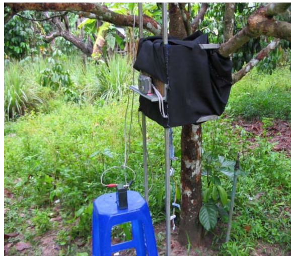
Figure A-2 Image Acquisition setting box control sunshine with Longkong fruit-clusters and PowerShot A20
