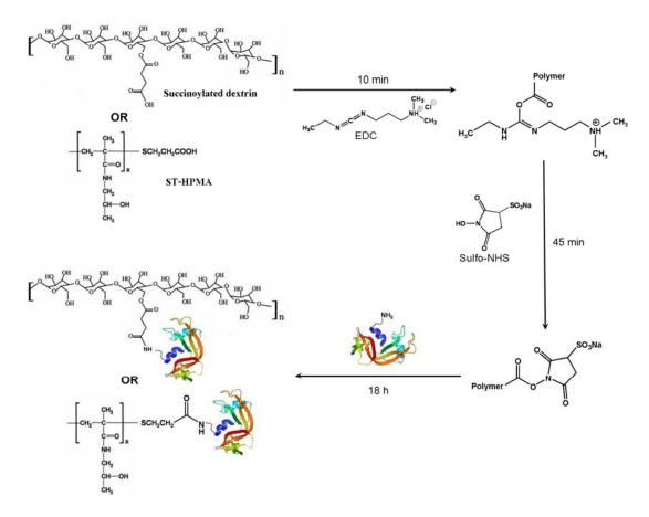
Figure 6.1 Reaction scheme for synthesis of polymer-RNase A conjugate
