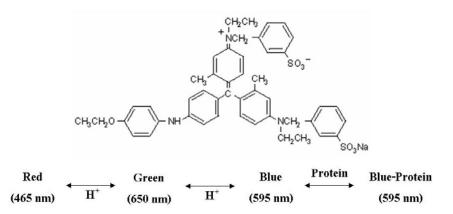
Figure 2.5 Structure of Coomassie blue G-250 dye and mechanism of Bradford assay (from Bradford, 1976).
