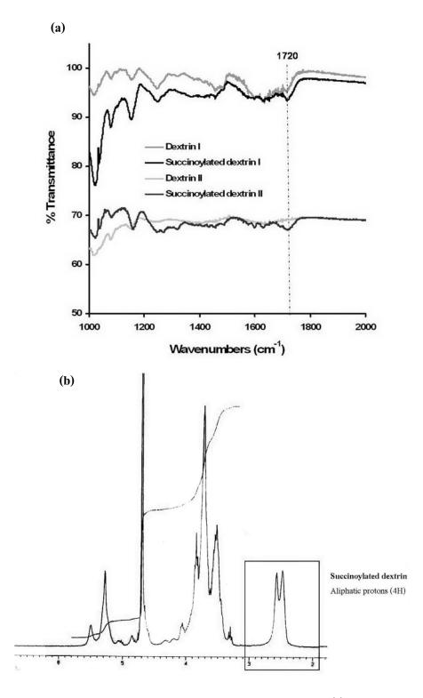
**Figure 5.6** Characteristics of dextrin and succinoylated dextrin. Panel (a) FT-IR of dextrin and succinoylated dextrin and panel (b)  $^{1}$ H NMR (D<sub>2</sub>O) spectrum of succinoylated dextrin.
