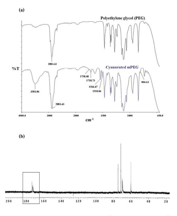
**Figure 3.6** Characterization of cyanurate mPEG using panel (a) FT-IR spectroscopy and Panel (b) <sup>13</sup>C-NMR.
