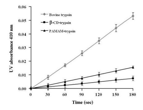
**Figure 4.6** Comparison of the enzymatic activity of the  $\beta$ -CD- and PAMAM-trypsin conjugates and native trypsin. In each case 2 mg/mL trypsin equivalent was used (mean ± SD, n=3).
