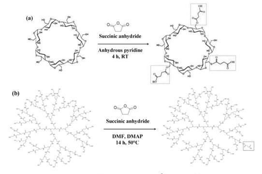
Figure 4.1 Reaction scheme for (a) succinoylation of  $\beta$ -CD and (b) succinoylation of the PAMAM dendrimer.
