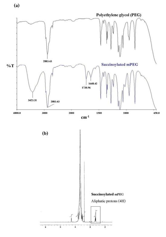
**Figure 3.5** Characterization of succinoylated mPEG using panel (a) FT-IR spectroscopy and panel (b) <sup>1</sup>H-NMR.
