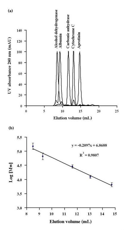
**Figure 2.2** FPLC analysis using Superdex HR 10/30 FPLC column. Panel (a) the FPLC chromatogram of protein molecular weight standards and panel (b) represents the calibration curve plotted to estimate molecular weight of sample.
