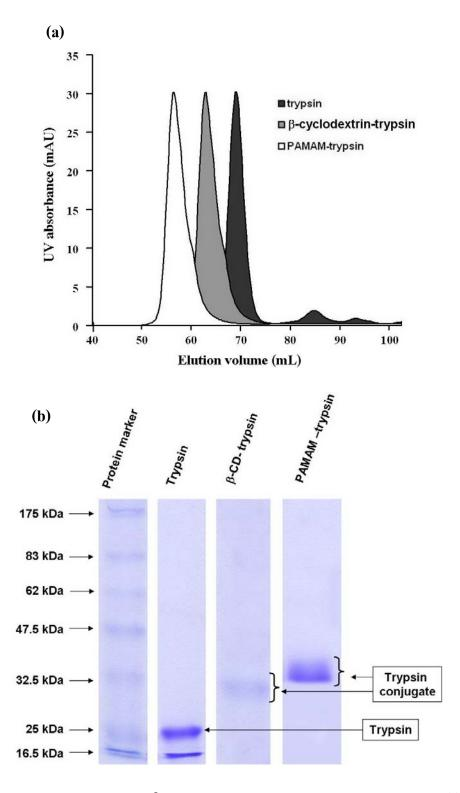
**Figure 4.5** Characterization of  $\beta$ -CD- and PAMAM-trypsin conjugate. Panel (a) FPLC chromatogram, and panel (b) SDS-PAGE electrophoresis.
