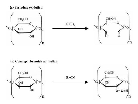
**Figure 5.2** Methods used for polysaccharide functionalization. Panel (a) periodate oxidation, (b) cyanogen bromide activation, (c) chloroformate activation, (d) succinoylation, and (e) tosylation.
