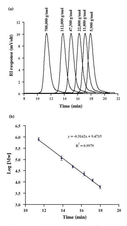
**Figure 2.3** GPC analysis of pullulan molecular weight standards (a) shows the chromatogram of the pullulan standards and (b) shows the calibration curve plotted using the Polymer Laboratories software, to estimate molecular weight and polydispersity of sample.
