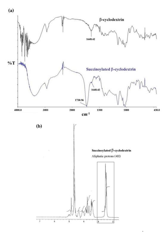
**Figure 4.3** Characterization of succinoylated  $\beta$ -CD. Panel (a) FT-IR and panel (b) <sup>1</sup>H-NMR. The spectra are compared to their parent polymer.
