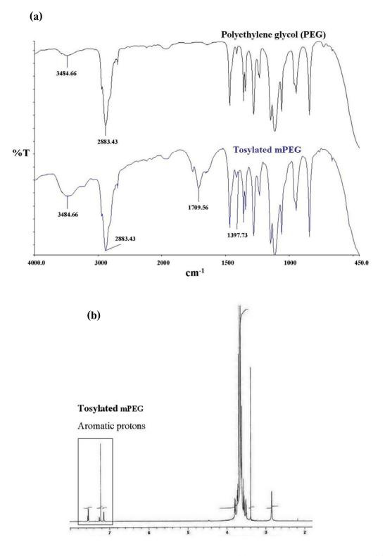
**Figure 3.7** Characterization of tosylated mPEG using panel (a) FT-IR spectroscopy and Panel (b) <sup>1</sup>H-NMR.
