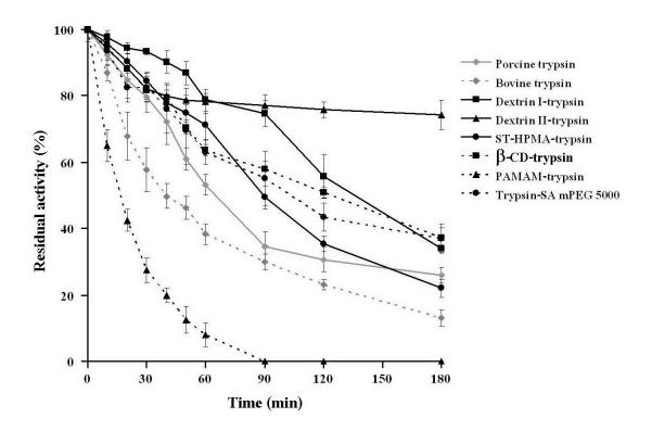
**Figure 5.13** Comparison of autolysis at 40 °C and activity of trypsin, and the dextrin I-, dextrin II-, ST-HPMA-,  $\beta$ -CD-, PAMAM- and PEG-trypsin conjugates. Activity was measured using BAPNA as a substrate (mean ± SD, n=3).
