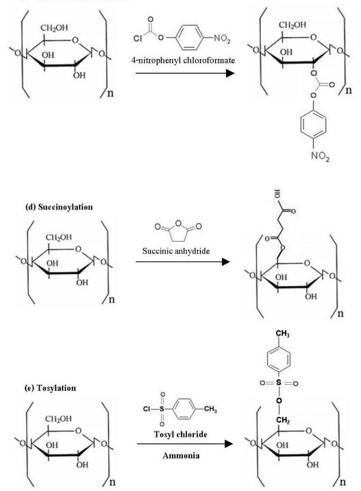
**Figure 5.2 Contd.** Methods used for polysaccharide functionalization. Panels (a) periodate oxidation, (b) cyanogen bromide activation, (c) chloroformate activation, (d) succinoylation, and (e) tosylation.
