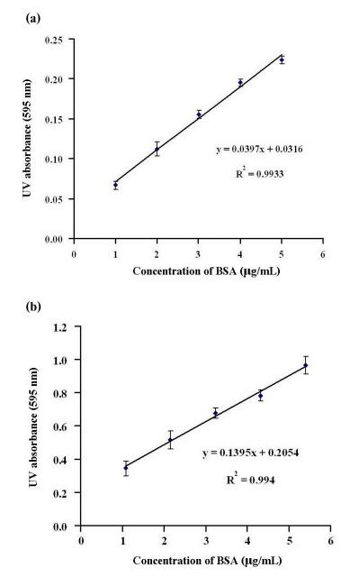
Figure 2.6 Bradford assay calibration curve using (a) a Hewlett Packard 8452A Diode array spectrophotometer (Ontario, Canada) or (b) a Sunrise UV-vis absorbance plate reader (Tecan, Austria)
