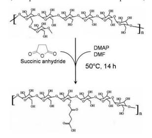
Figure 5.4 Reaction scheme for synthesis of succinoylated dextrin
