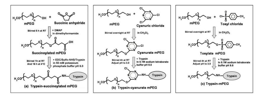
**Figure 3.4** Reaction for synthesis of PEG-trypsin conjugates. Panel (a) Trypsin-succinoylated mPEG, panel (b) Trypsin-cyanurate mPEG and panel (c) Trypsin-mPEG conjugate (taken from Treetharnmathurot et al., 2008).
