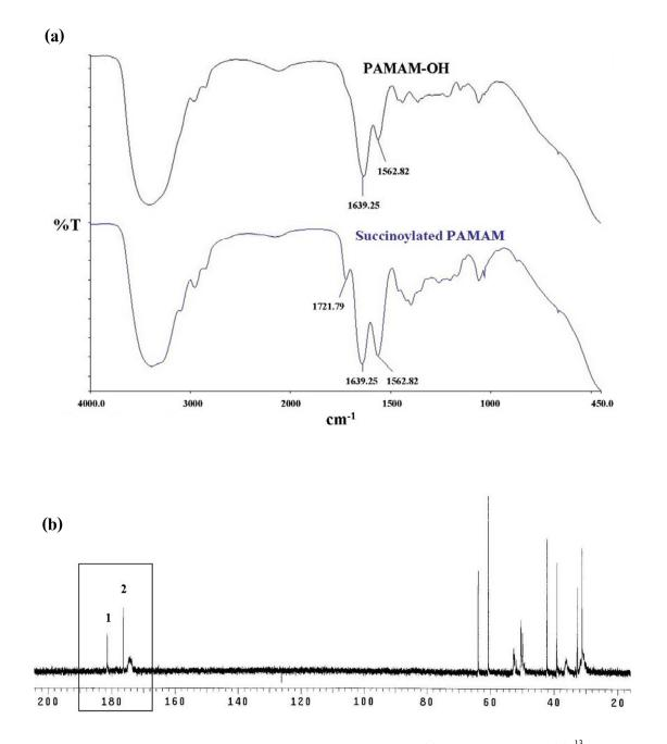
**Figure 4.4** Characterization of succinoylated PAMAM. Panel (a) FT-IR and panel (b) <sup>13</sup>C-NMR spectrum; peak (1) is carbonyl of carboxylic at 181.4 ppm and peak (2) is carbonyl of ester at 176.3 ppm. The spectra are compared to their parent polymer.
