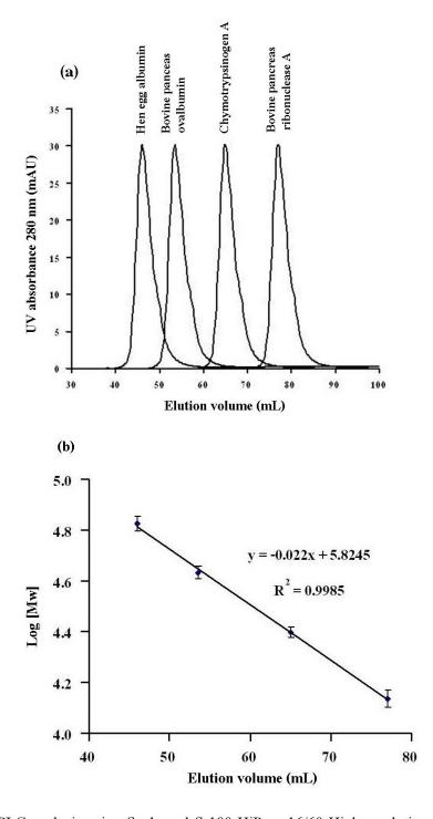
**Figure 2.1** FPLC analysis using Sephacryl S-100 HiPrep 16/60 High resolution FPLC column. Panel (a) the FPLC chromatogram of protein molecular weight standards and panel (b) the calibration curve obtained by plotting Log molecular weight against elution volume to estimate molecular weight of sample.
