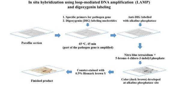
**Figure 11.** Procedure of *in situ* hybridization using loop-mediated DNA amplification with digoxigenin labeling (ISDL)
