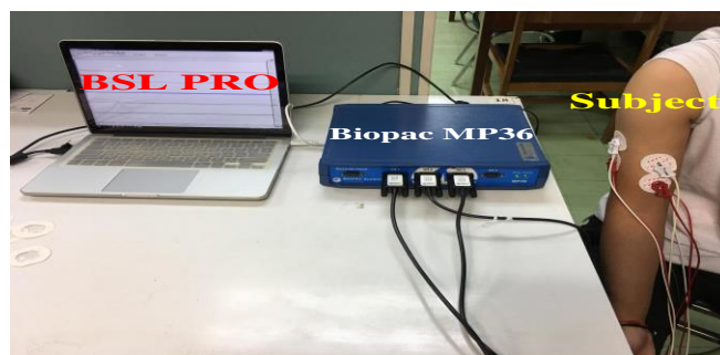
Fig. 3.10 The complete signal measurement system
