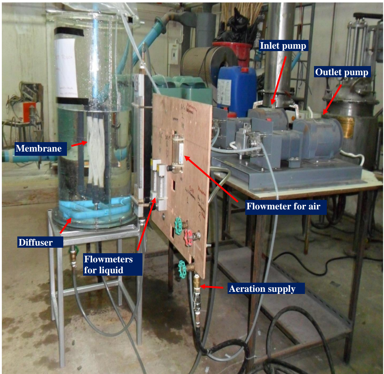
Figure 3.2 Laboratory setup of MBR.
