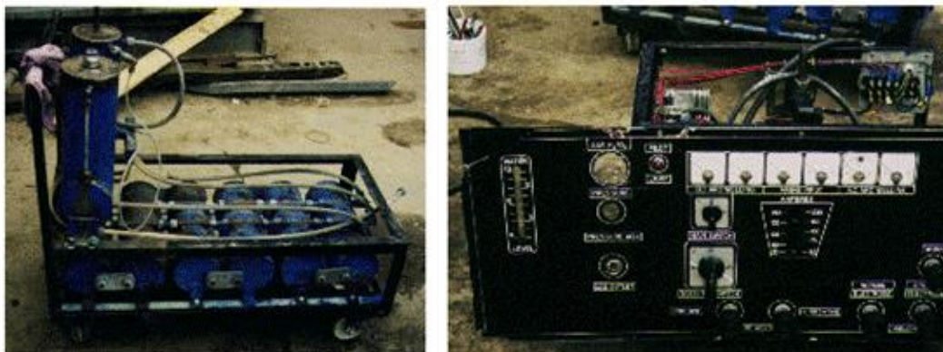
Figure 5 Multi-HHO generator unit (Left) and system controller (Right) [33].
