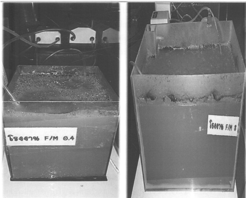
Figure 37 Comparison wastewater treatments using sludge from aerobic pond of E-Hub Huad Company between F/M ratio as 0.4 and 8 mg-COD/mg-MLVSS/d at DO 2 mg/L, OLR of 2 g-COD/L/d and HRT of 10 day
