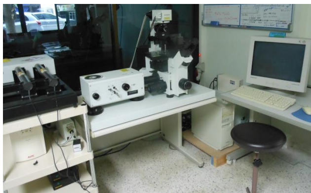
Fig. 5 Demonstrating confocal laser scanning microscope (CLSM) (FV300, Olympus, Japan) used to examine fluorescence live-dead staining of cells on titanium disks.
