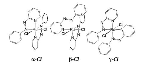
Structural representation of (the  $\Delta$  enantiomers of)  $\alpha$ -[Ru-(azpy)<sub>2</sub>Cl<sub>2</sub>] (left),  $\beta$ -[Ru(azpy)<sub>2</sub>Cl<sub>2</sub>] (middle) and  $\gamma$ -[Ru(azpy)<sub>2</sub>Cl<sub>2</sub>] (right). (*Inorg. Chem.* 2000, **39**: 2966-2967.)
