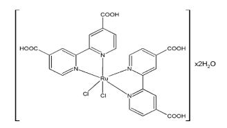
Molecular configuration for the [Ru(II)(dcbpyH<sub>2</sub>)<sub>2</sub>Cl<sub>2</sub>]·2H<sub>2</sub>O complex. (*J. Mat.Pro.Tech.* 2005, **161**: 234-240.)
