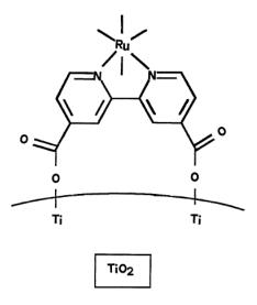
Adsorption of Ru-bpy sensitizes on TiO<sub>2</sub> particles via formation of ester-like linkages. (*Sol. Energy Mater, Sol. Cells*. 1998, **53**: 163-175.)
